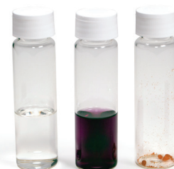
Figure 9. Left to right: CBD before Beam test; HU-331 after Beam test; crystalline HU-331.
